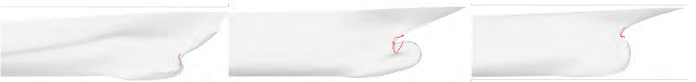
Figure 23: Examples of invalid (self-intersecting) designs resulted from the GAN model. The red curve indicates the regions of intersection.
