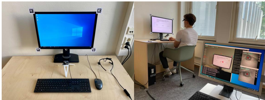
Figure 2. Left) Monitor with apriltags, Pupil Core to the right, and microphone in the middle. Right) Experimenter monitors eye-tracking real time during experimental run.
